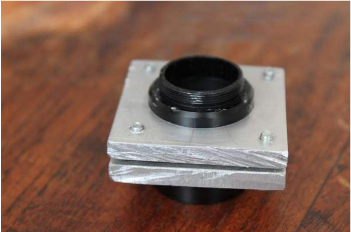
Finished – CS mount – screws direct into DMK
