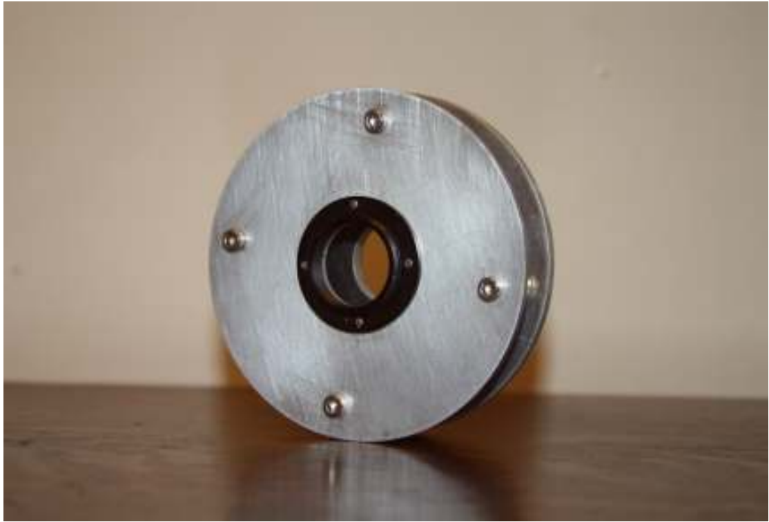
Assembly showing male C mount flange.
